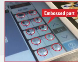
The protective sheet (free operation display) on touch panel is embossed. Since it has a touch feel, incorrect input can be prevented.
